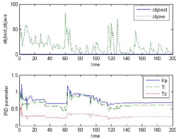
Fig. 16. Search process for optimal parameter values of an AVR system by GA–BF method for  $\beta = 1.0$ .
