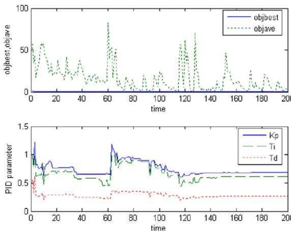
Fig. 15. Search process for optimal parameter values of an AVR system by GA–BF method for  $\beta = 0.5$ .
