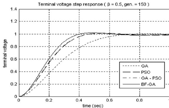
Fig. 12. Terminal voltage step response of an AVR system with different controllers ( $\beta = 0.5$ , generations = 200).
