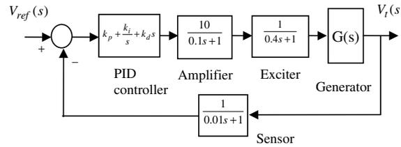
Fig. 9. Block diagram of an AVR system with a PID controller.
