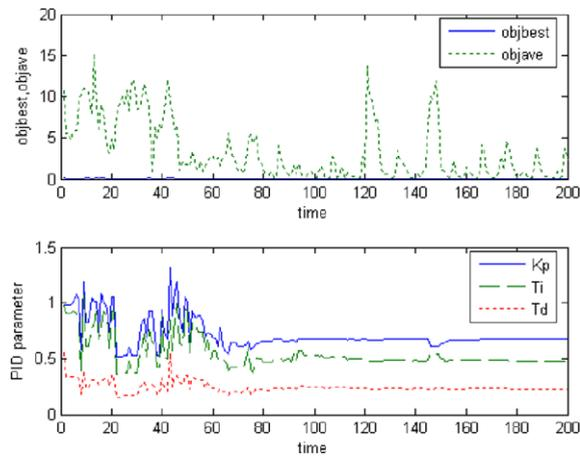
Fig. 17. Search process for optimal parameter values of an AVR system by GA–BF method for  $\beta = 1.5$ .
