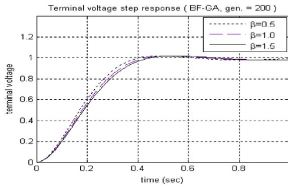
Fig. 11. Terminal voltage step response of an AVR system using GA–BF algorithm.
